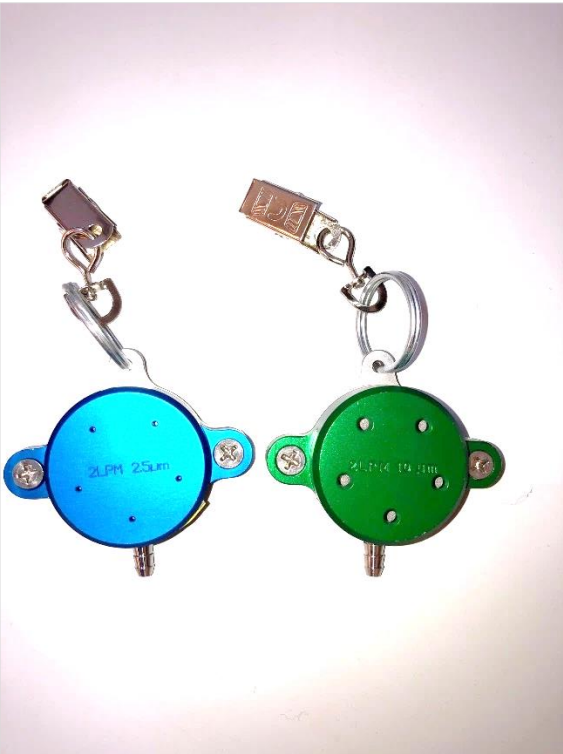
Figure 2. Impactor Heads to monitor PM 2.5 and PM 10 aerodynamic diameter dust fraction size.
